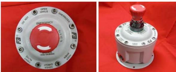
RJB11S2001 Emergency Stop. The robust external operator can be removed only with a special tool and can withstand shocks, impacts and vibrations as required by IEC60947-5-5. Latching operator, twist-to-release. Key release, locking and guard options available.
