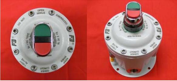
RJB11S2008 Key Switch and RJB11S2009, RJB11S2010 Selector Switches. Available in a variety of configurations: 0-1, 1-2, 1-0-2, 1-2-3, AUTO-MAN, FWD-OFF-REV etc. Up to 2 separate contacts available in each position. Choice of silver 690Vac or gold quad-connect low voltage contacts.
