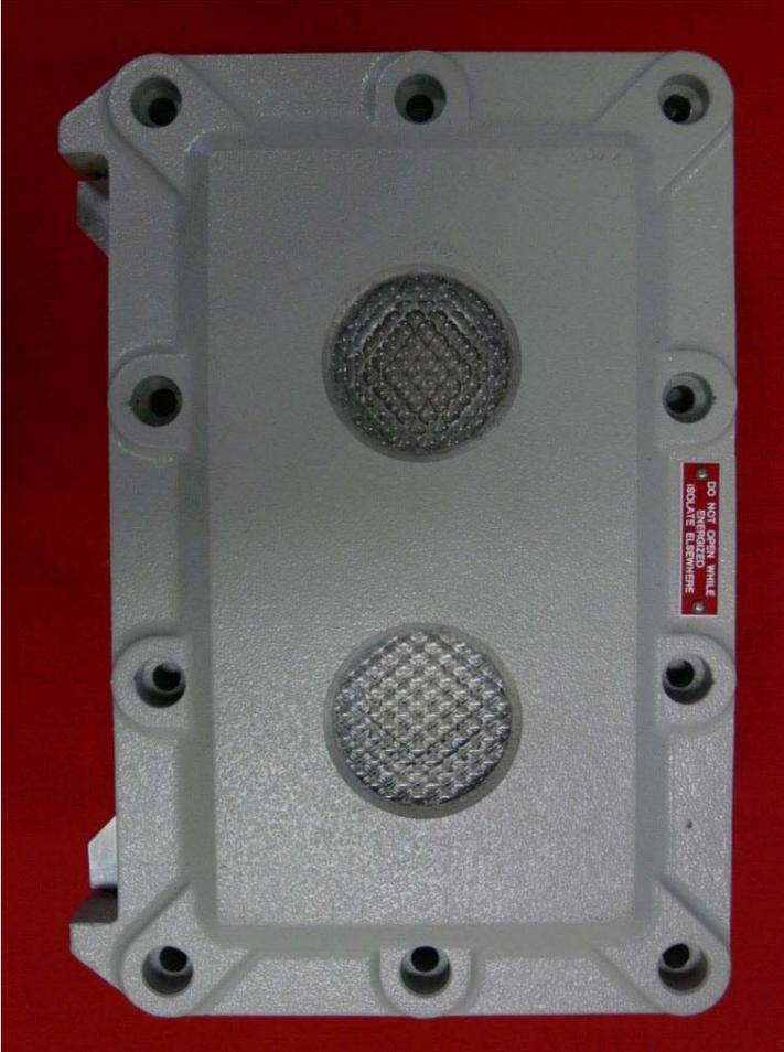
We offer LED lighting solutions in the FJB enclosures. The cool, highly efficient operation is flicker-free and never requires lamp replacement. Various power and luminous intensity are available in each size, with dimmable control and emergency options. EXIT signs etc also available. These light fittings are suitable for the most demanding applications in hazardous areas (zone 1 Ex d+H2 T6, zone 21 T85/T100C, IP66/IP67), corrosive and saline environments.
