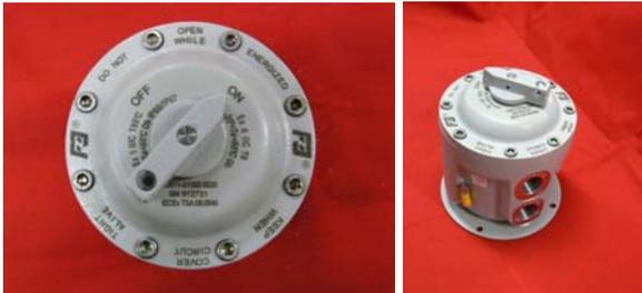
RJB11S1500 isolator and selector switches up to 4p 32A 11kW AC3. Feature padlockable handle, cable entries in the bottom side or top-bottom. Mounting base with 4 fixing points. External equipotential bonding connection facility for 4-6 mm<sup>2</sup> wire.
